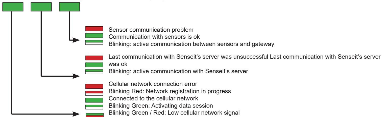
Note 1: The cellular gateway resets itself after receiving new configuration from the server (ex. new HB), the LEDs will change colors briefly, then each LED will flash red as the gateway connects. When all LEDs have turned green, the reset cycle has completed.
