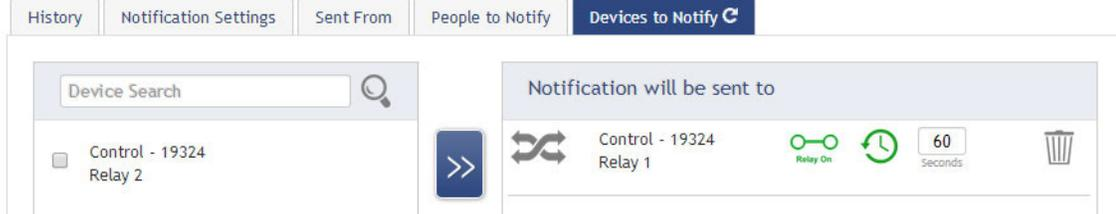
**Note:** Control devices have two relays per device that are controlled separately. You can turn a relay on, off or toggle the state. You can also set a duration by clicking on the timer icon. This will perform the selected toggle (on/off/toggle) for a set duration, then change back.
