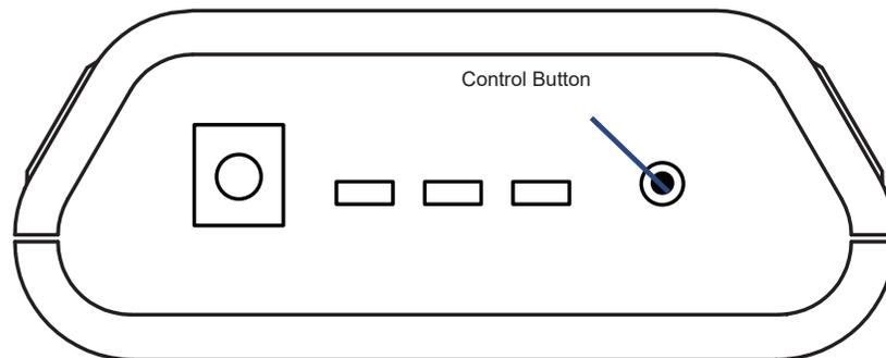
A short press of the control button while lights are all green, will force immediate communication to server and exchange all sensor data currently stored in memory.
